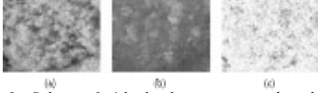
Figure 1. Subset of 4-look slant range radar data: (a) intensity, (b) interferometric z-coordinate, and (c) coherence magnitude for track KAL.17A.
